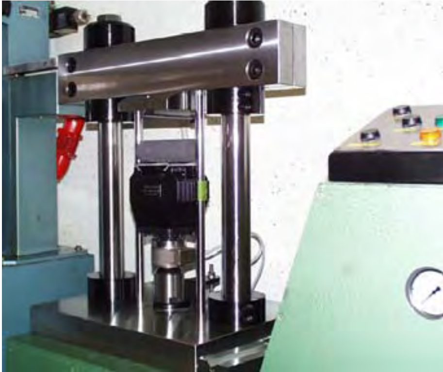
Figure 6: Apparatus for testing anode samples.
