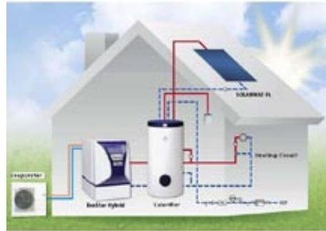
**Figure 11:** Function of air source heat pump
