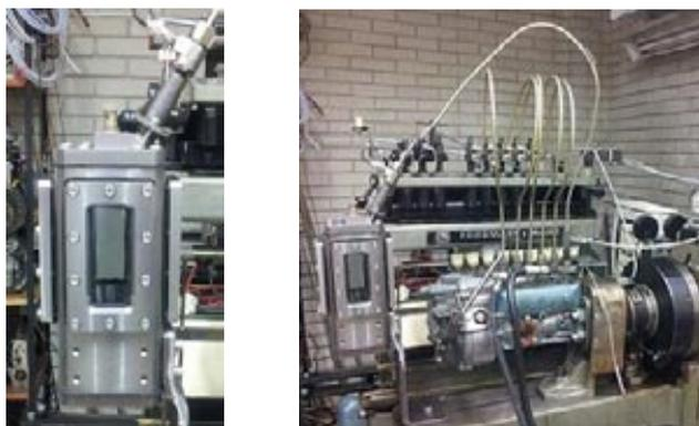
**Figure 2:** Experimental setup – pressure chamber and Friedmann & Maier fuel injection system
