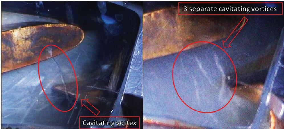
**Figure 3:** Cavitating vortices in the distributor region
