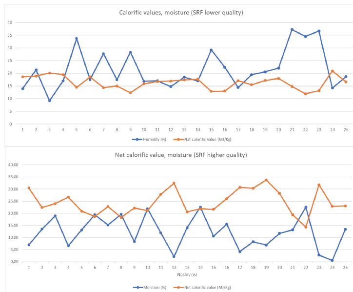
Figure 2: Calorific values compared to the moisture content of individual fuel samples of lower quality (up) and higher quality (down)
