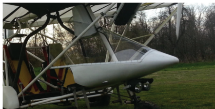
Figure 17: Installed manufactured open cabin
