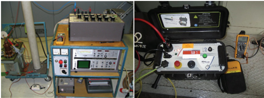
Figure 6: Tan \delta testing equipment with 50Hz (left) and 0.1Hz frequency
