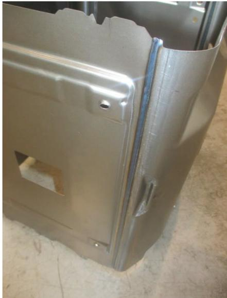
**Figure 12:** An example of welded U-circumference and front end, [7]
