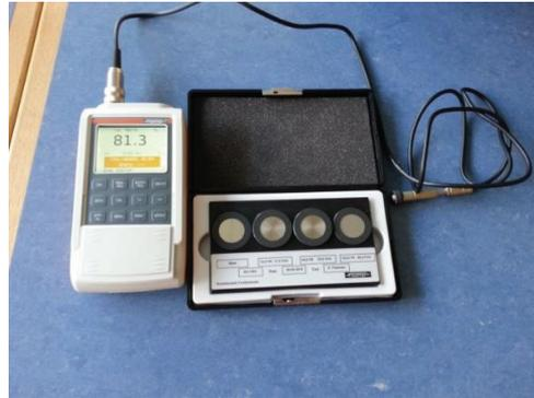
**Figure 1:** Calibrating of ferritoscope device Fisher with calibration samples, [5]
