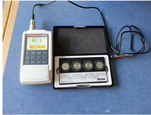
Figure 1: Calibrating of ferritoscope device Fisher with calibration samples, [5]
