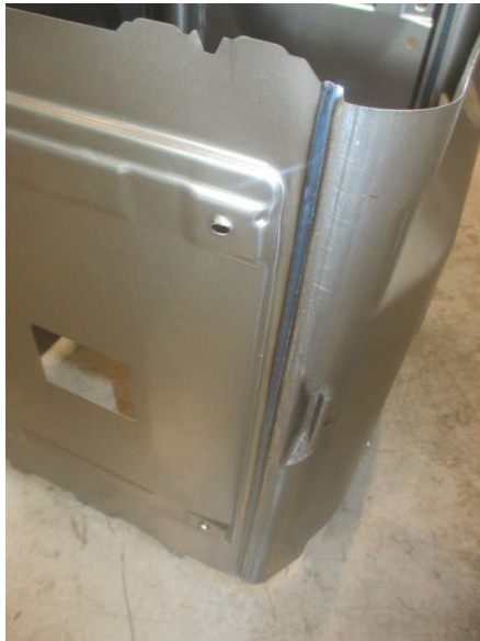
Figure 12: An example of welded U-circumference and front end, [7]
