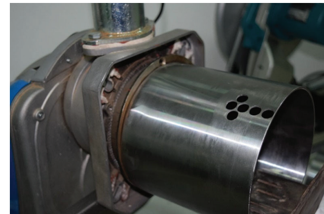
Figure 11: Cr-Mo steel tube with damaged surface (6 holes) of 5.70 cm 2
