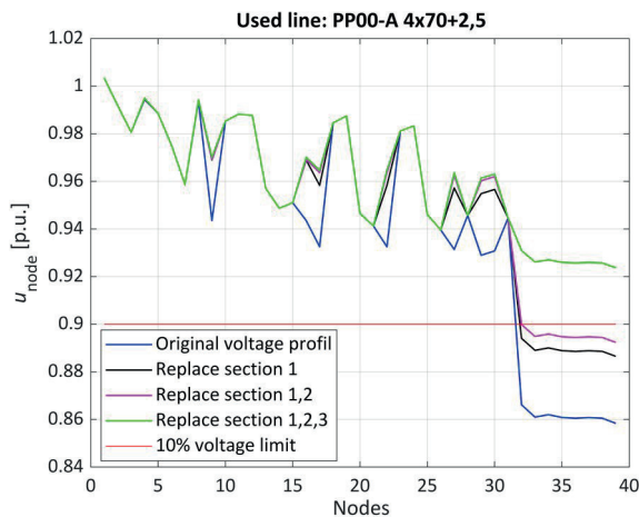
Figure 17: Voltage profile with conductor type PP00-A 4x70+2.5 in selected sectors
