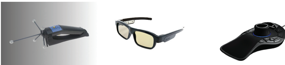
Figure 8: Interaction devices: Wand, Master Shutter glasses and 3D SpaceMouse
