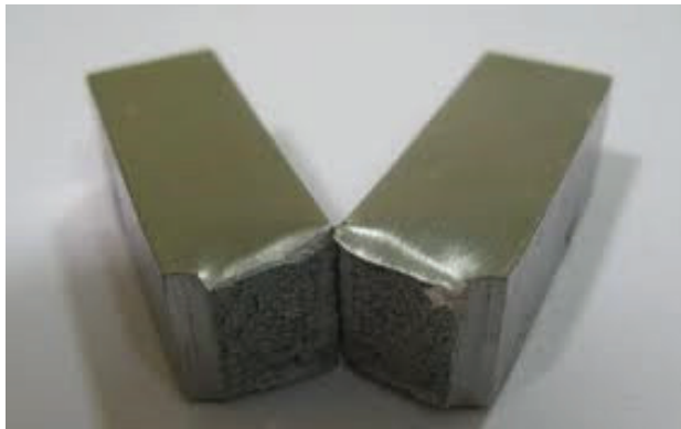
Figure 4: The appearance of the groundbreaking surface of the Charpy sample
