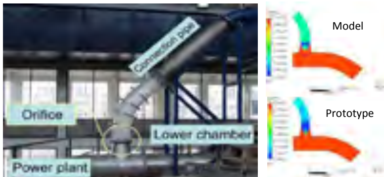
Figure 9: Scale Model of pipe junction (left) and numerical model of nozzle (right) [7].
