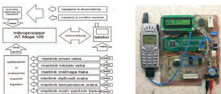
Figure 2: Electronic part of the meteorological station (Korošec L., Tržan S.)
