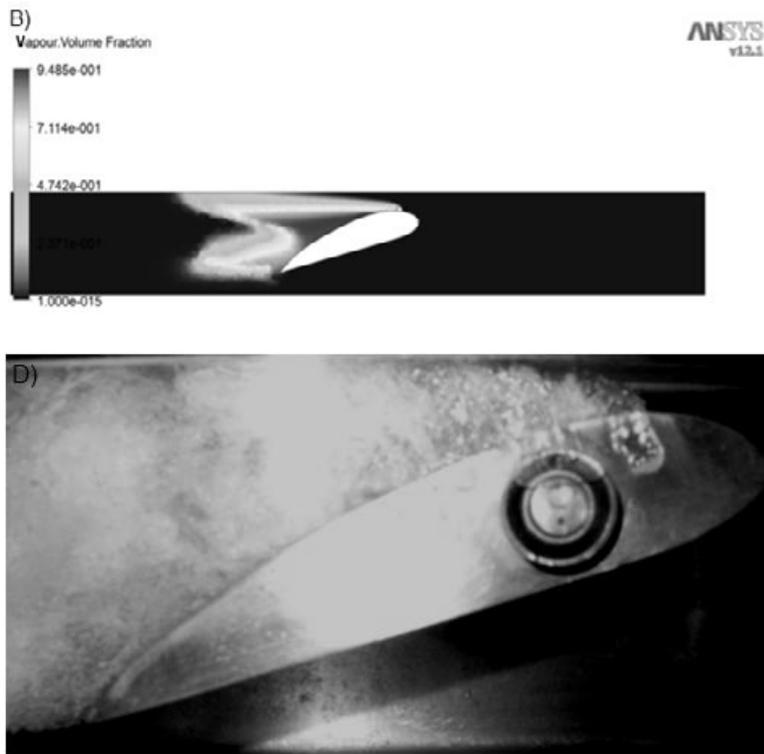
Figure 4: Comparison of simulations of the vapour phase of the experiment
