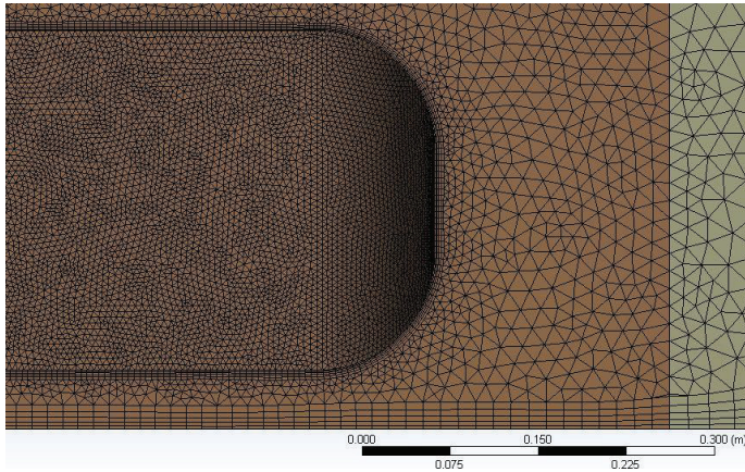
Figure 4: Detail of numerical mesh near Ahmed body
