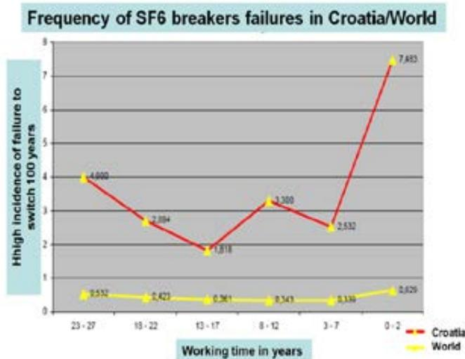
**Figure 3:** SF<sub>6</sub> Breakers failures in Croatia/World
