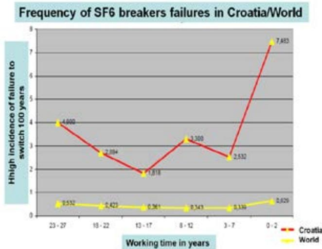
**Figure 3:** SF<sub>6</sub> Breakers failures in Croatia/World
