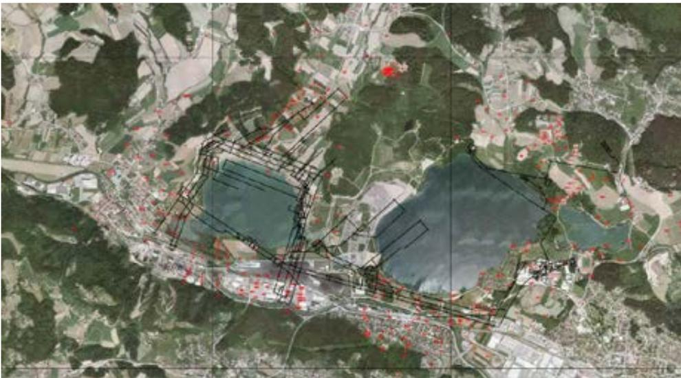
**Figure 1:** A broader area of the Velenje Coal Mine showing the mine roadways (black) and points of observation networks on the surface (red).
