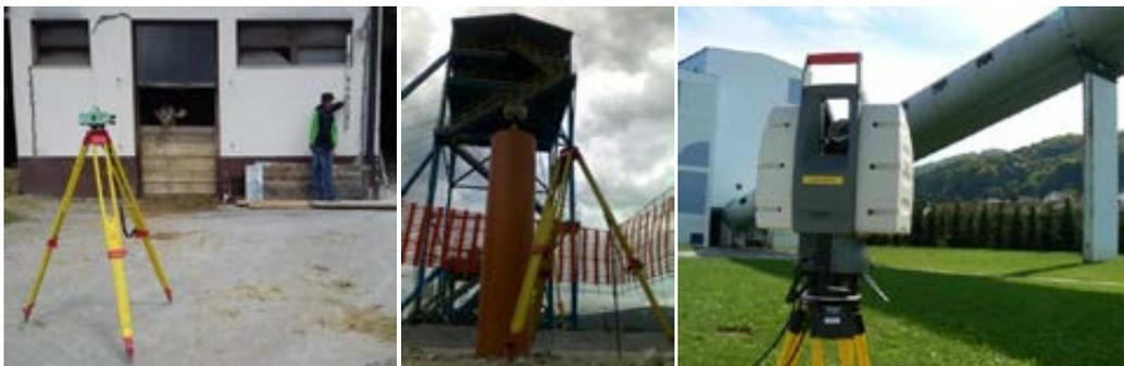
**Figure 4:** Monitoring the movements on a building with: the method of geometric levelling (left), the static GNSS measurement (middle), the use of a 3D terrestrial laser scanner (right).
