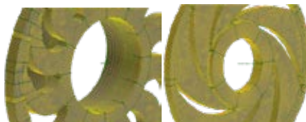
Figure 4: CV mesh of stator (left) and rotor (right).
