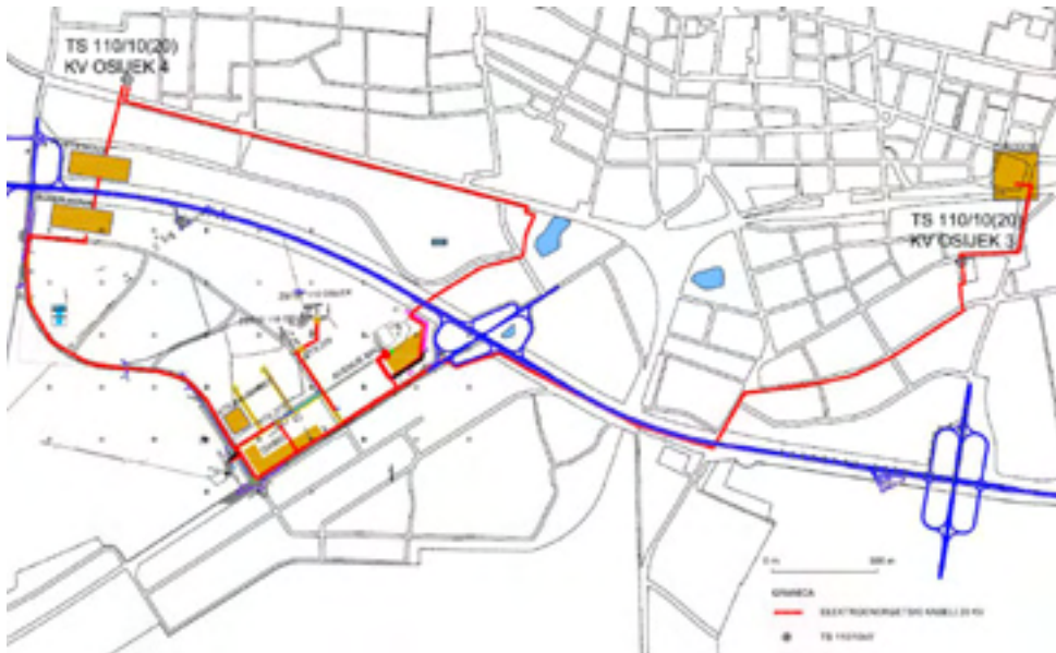
Figure 6: Plan of 20 kV electricity distribution network of the city (red line is a new 20 kV high voltage cable, blue line is a city of Osijek detour road)
